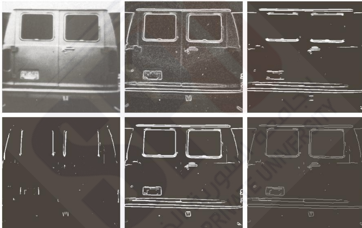
FIGURE 10.27 (a) A 534 \times 566 image of the rear of a vehicle. (b) Gradient magnitude image. (c) Horizontally connected edge pixels. (d) Vertically connected edge pixels. (e) The logical OR of the two preceding images. (f) Final result obtained using morphological thinning. (Original image courtesy of Perceptics Corporation.)
