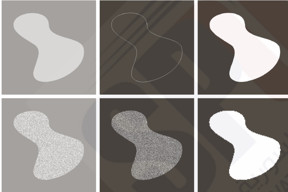
FIGURE 10.1 (a) Image containing a region of constant intensity. (b) Image showing the boundary of the inner region, obtained from intensity discontinuities. (c) Result of segmenting the image into two regions. (d) Image containing a textured region. (e) Result of edge computations. Note the large number of small edges that are connected to the original boundary, making it difficult to find a unique boundary using only edge information. (f) Result of segmentation based on region properties.
